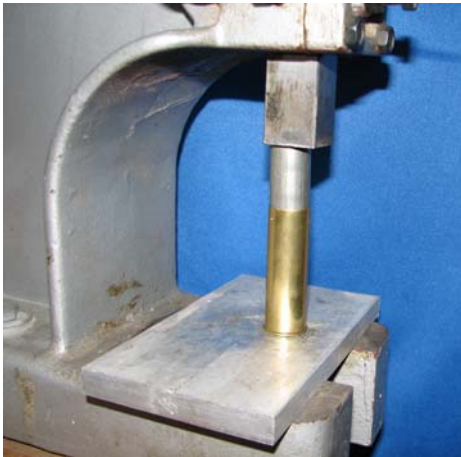
Using arbor press & Lee Load-all II to square overshot wads
