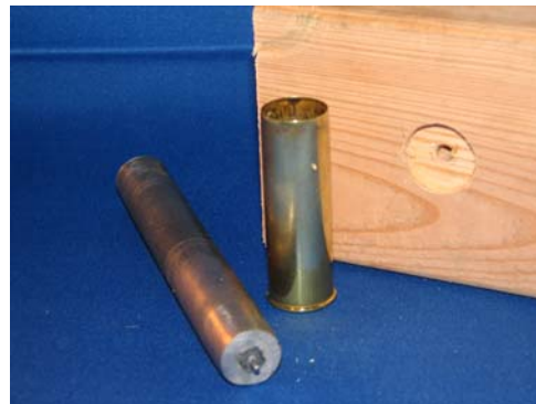
De-priming tool, shell and wood block drilled on both sides
