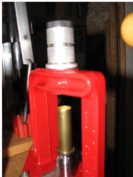
Using arbor press & Lee Load-all II to square overshot wads
