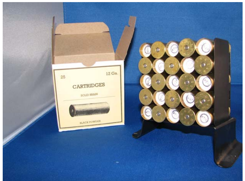
Finished shells on Horandy shell stacker ready to be put in box
