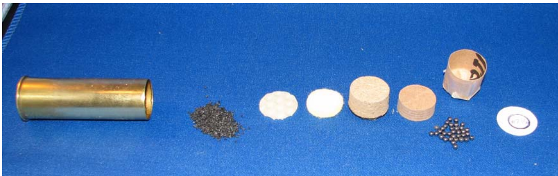
Brass shell, black powder, beeswax wad, felt wad, 1/2" and 1/4" filler wads, shot, homemade shot cup and over shot wad
